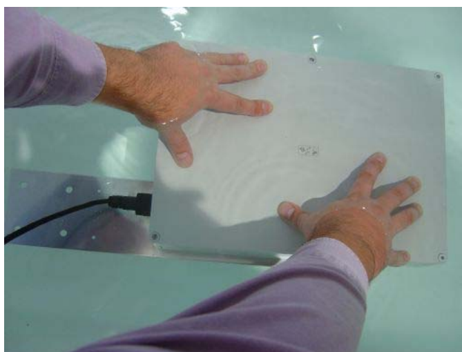
Submersed - XWLAN UAP3 IP66 rated enclosure and connectors.
